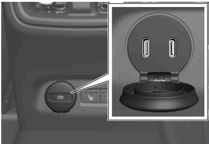
USB-poorten (type C) in tunnelconsole, achterbank.
