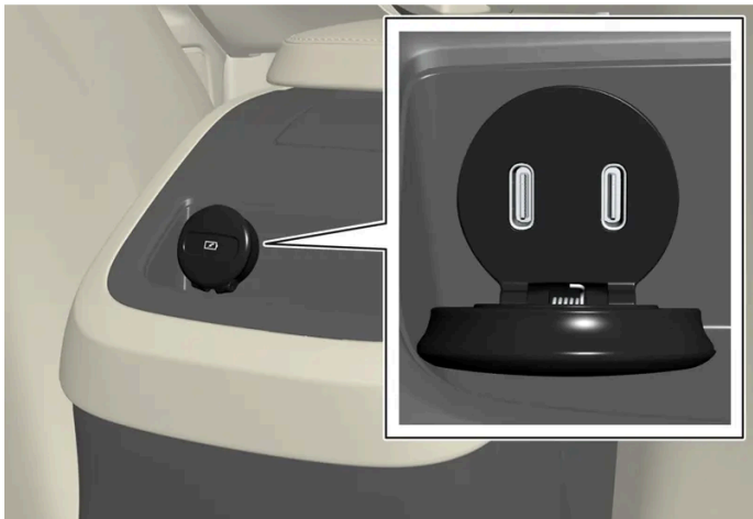
USB-poorten (type C) in tunnelconsole, achterbank.
