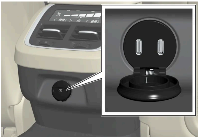
USB-poorten (type C) in tunnelconsole, achterbank.
