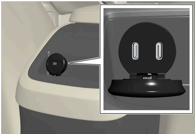
USB-poorten (type C) in tunnelconsole, achterbank.
