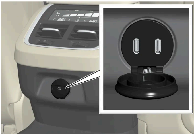
USB-poorten (type C) in tunnelconsole, achterbank.
